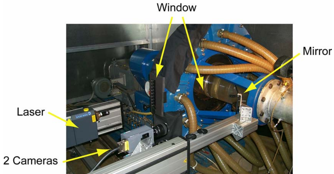
Figure 38: Picture of Test Rig for Combined PIV Measurements and Cavitation Observation.
